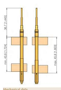
The VF 5 is mounted in the KS-VF5 030
